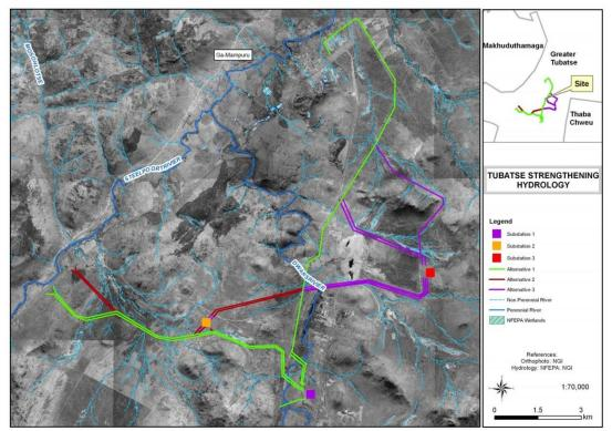
**Figure 3:** The hydrology of the general area targeted for a new substation on one of three alternative sites, and accompanying high tension power lines. The relief discernable on the map amply illustrate that the power lines are indeed planned to skirt mountains and the conservation area west of the proposed alternative site 3 for the substation.
