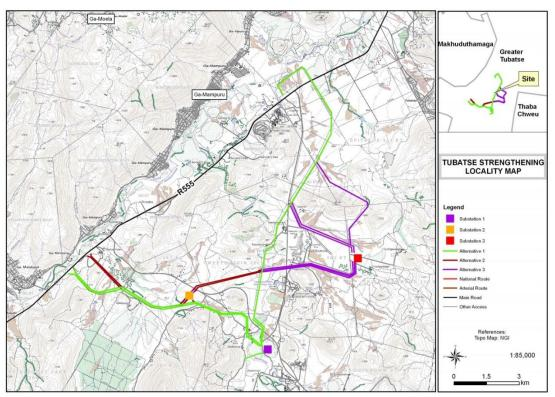
**Figure 2:** Topocadastral map illustrating the three proposed locations for the new substation, and the associated incoming and outgoing power lines that would connect it to the Senakanwedi Substation and to the end of the new (to be constructed) southwest orientated line parallel to the R555.
