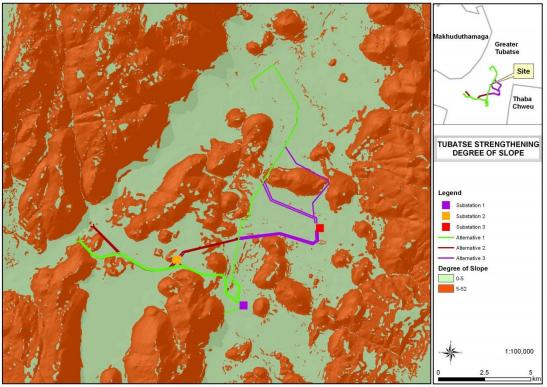
**Figure 1:** Map of the study area illustrating the fact that ESKOM avoided hillsides by routing the power line along the valley floor with a degree of slope 0 - 5°.
